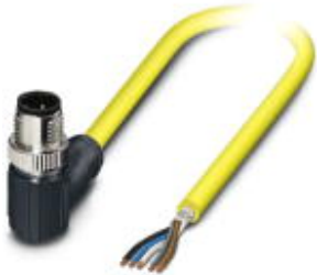
Sensor/Actuator cable, 5-position, PVC, Yellow RAL 1021, shielded, Plug angled M12-SPEEDCON, A-coded, on Free cable end, Cable length: 2 m
